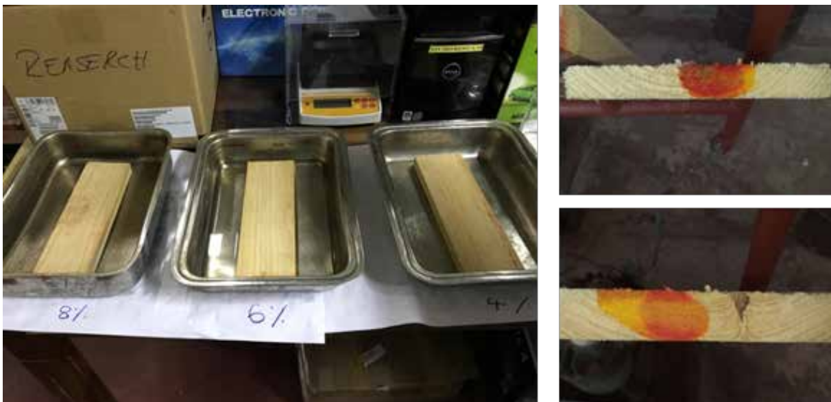
Conducting research on the effectiveness of different dipping periods of Boron for pine wood
